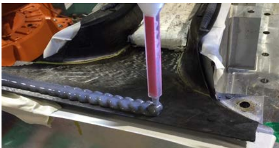
Figure 7-22. Adhesive Dispensing with Robot Head on Hat Prior to Assembly
