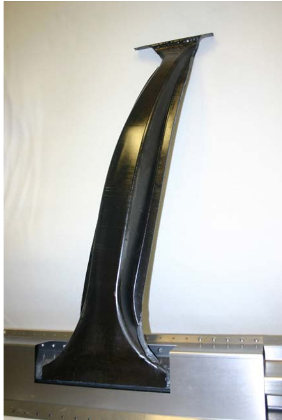
Figure 7-26. Adhesively Bonded Assembly of B-Pillar and Rocker
