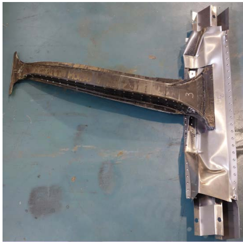
(a) Post-LVI Deformation and Damage
