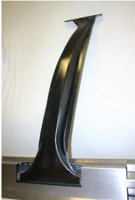
Figure 2-2. Adhesively Bonded Assembly of B-Pillar
