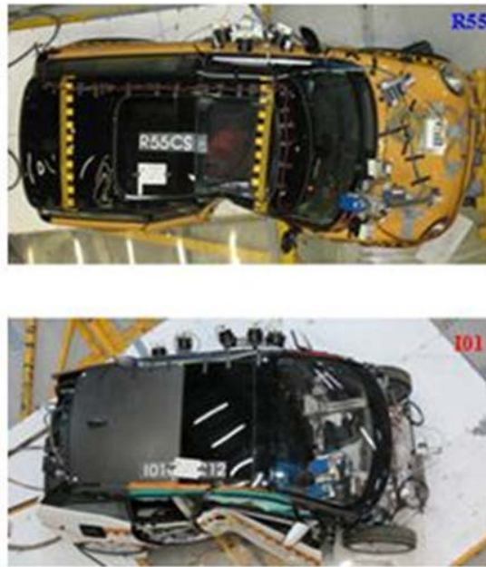
Figure 3-9. Occupant Compartment After Side-Impact, Steel (top) Versus CFRP (bottom)
