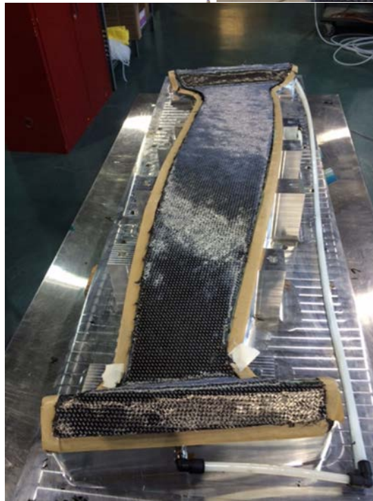
Figure 7-3. Preform Kitting and Assembly on Tool
