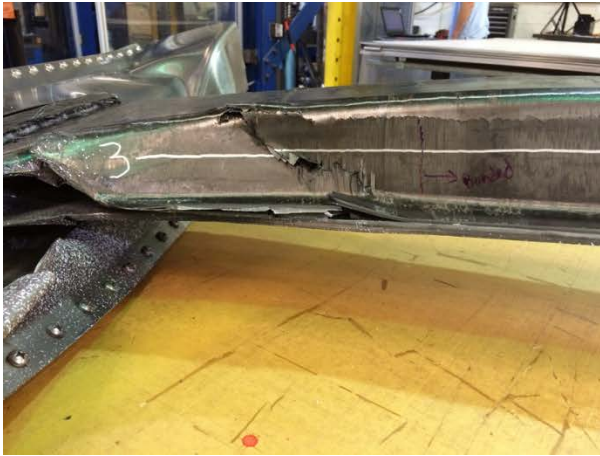
(a) Hat Crush and associated Web Fracture
