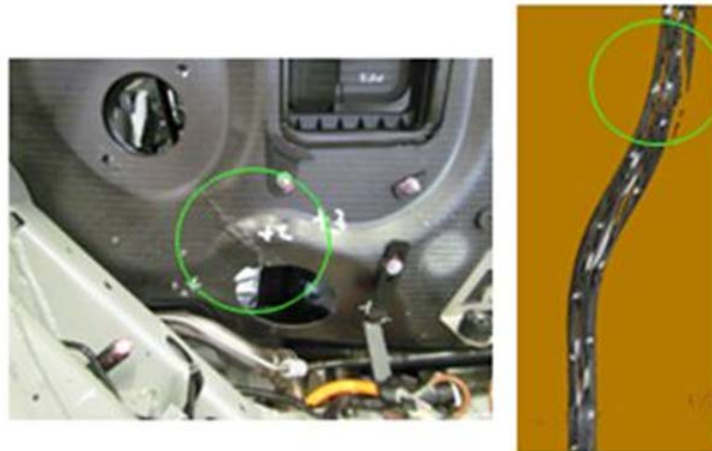
Figure 3-10. CT-Scan of Splintering in Bulkhead After Frontal Impact
