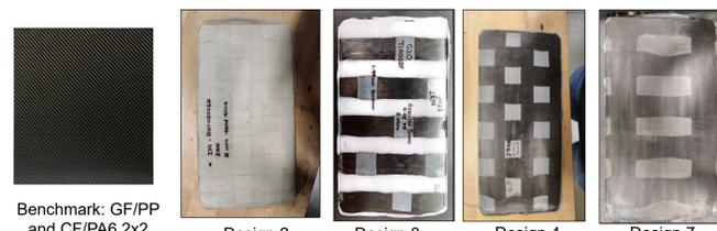
Figure 4 : Consolidated blanks with woven lattice reinforcement designs
