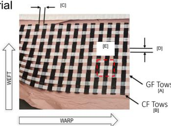
Figure 3 : Lattice Reinforcements
