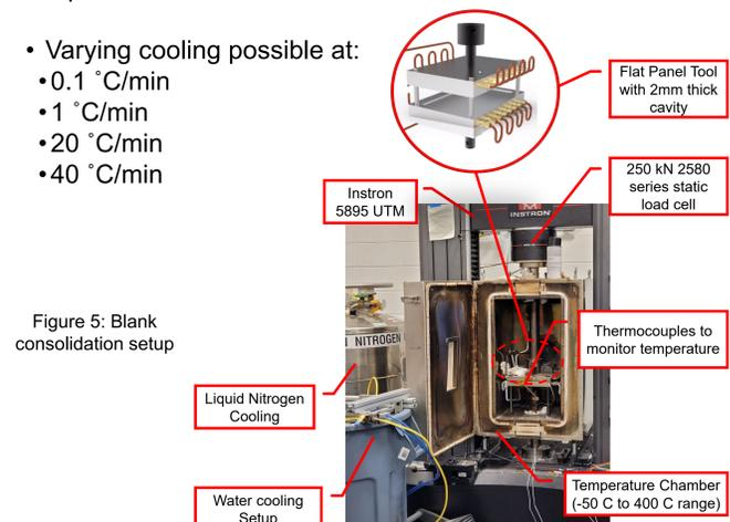
Figure 5: Blank consolidation setup
