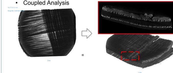
Figure 9: Micro CT evaluation of flex tested specimens before and after flex testing
