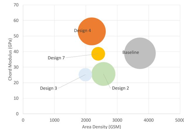
Figure 7: Chord Modulus v/s area density for various lattice designs
