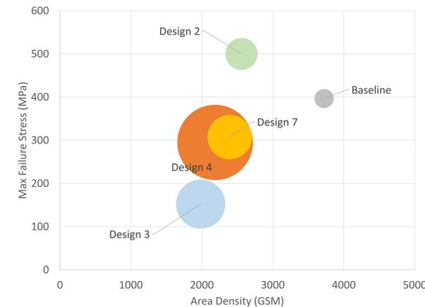
Figure 8: Max. Failure Stress v/s area density for various lattice designs
