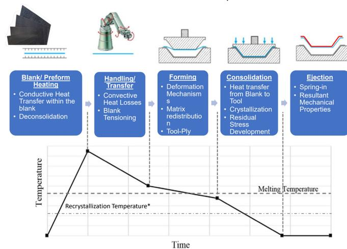
Figure 2: Thermoforming Process Discretized into distinct steps<sup>[5]</sup>
