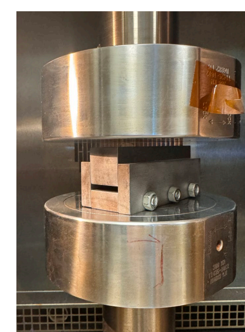
Figure 5: The fixture and sample heating for one hour between the compression grips of the Instron machine
