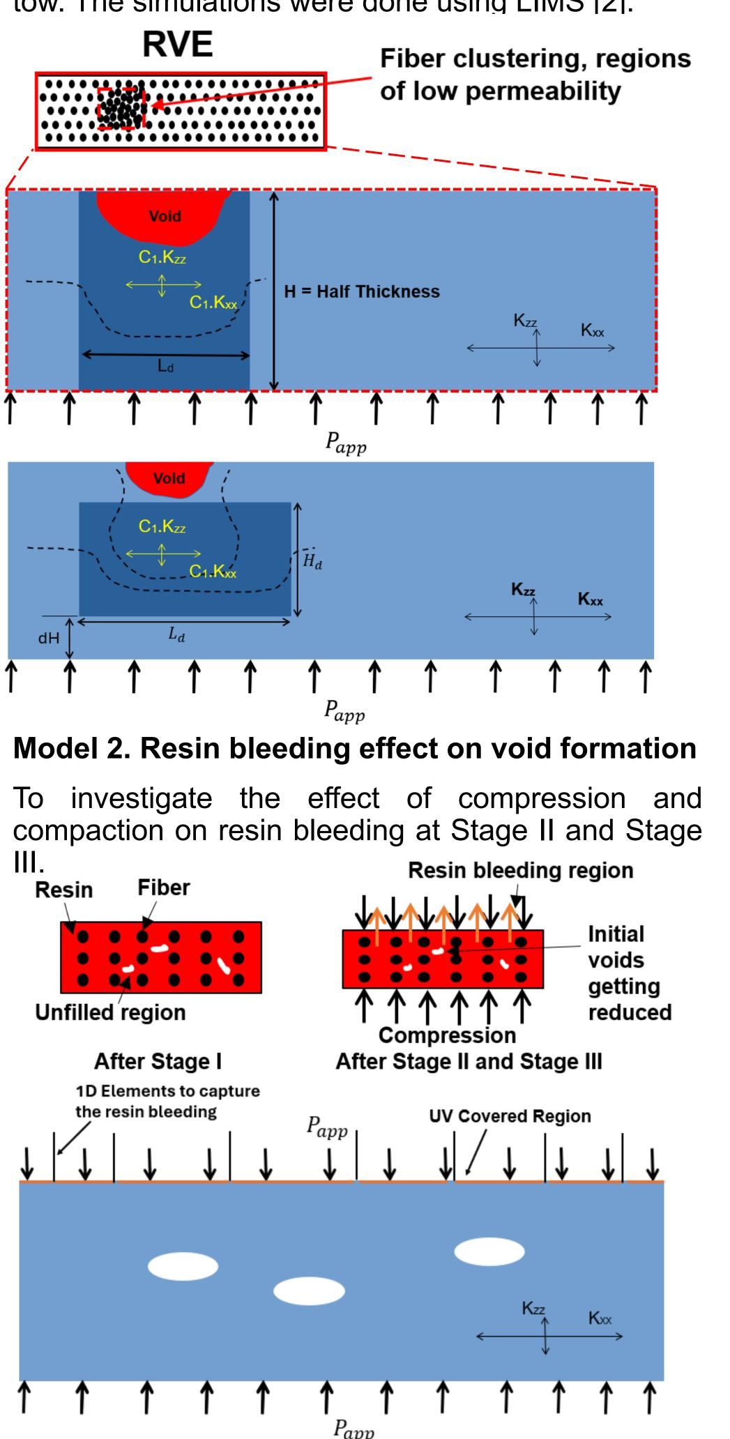
$C_1$  = Permeability variation factor =  $\frac{k_{low}}{k_{bulk}}$ ,  $L_d$  = length of the low permeability region (mm), dH = distance between the injection point and the low permeability region (mm), K = permeability  $(m^2)$ , P = Applied pressure (Pa)
