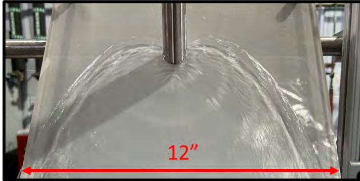
Water/Fiber jet on the spillway
