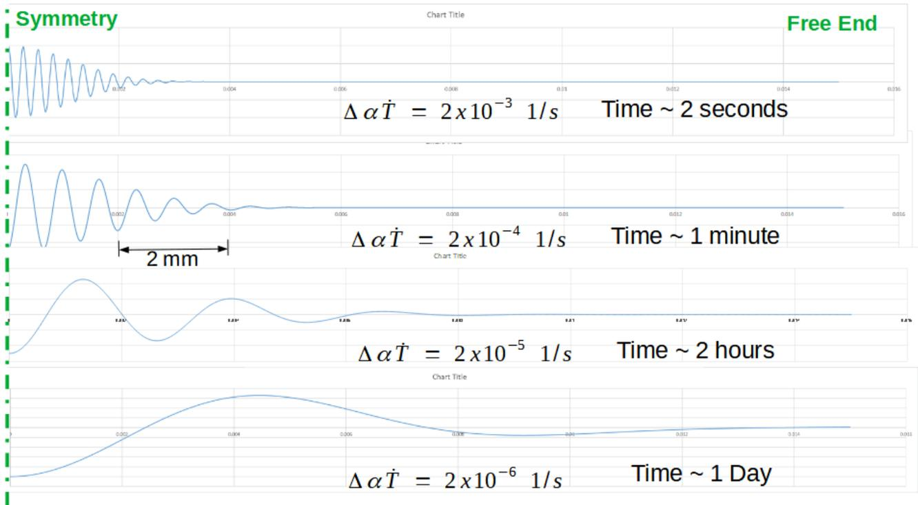
*Fiber buckling shape and time based on the rate of cooling: Viscosity constant.*
