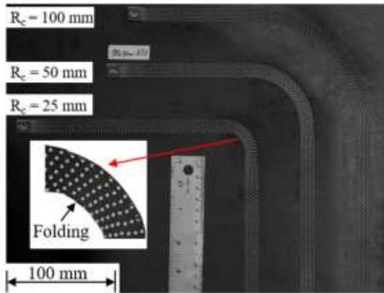
Steering of 12.5mm TuFF PEI tape at 100, 50 and 25 mm steering radius with applied tensile strains of 10, 18 and 32%, respectively.
