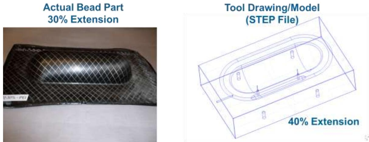
Formed Thermoplastic bead and the mold geometry.
