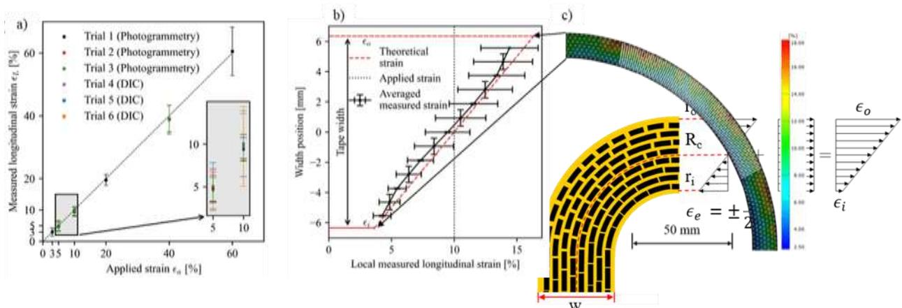
The measurements also confirm that when stretch-steering Tuff tape, the resulting strain across the tape width is the superposition of the in-situ applied tensile strain and in-plane bending computed from the tape width and steering radius.
