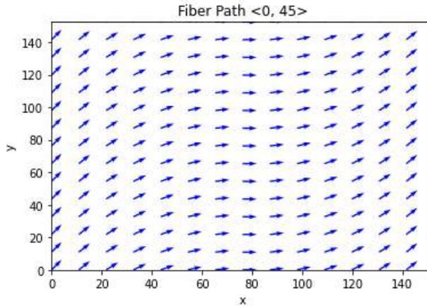
*Example of the implemented linear tow-steering path for a  $\langle T_0, T_1 \rangle = \langle 0, 45 \rangle$  ply, where  $T_0$  is the fiber angle at the center of the ply and  $T_1$  is the fiber angle at the ply edges.*
