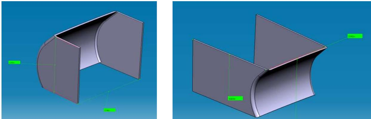
*Forward and Aft Loading Vanes from the reverser cascade assembly.
