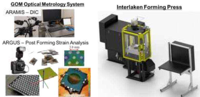
The Interlaken forming press was customized with a C-axis Sapphire sight glass, gas pre-heat system, and heated tool sets in order to conduct isothermal forming experiments with direct in-situ visualization.
