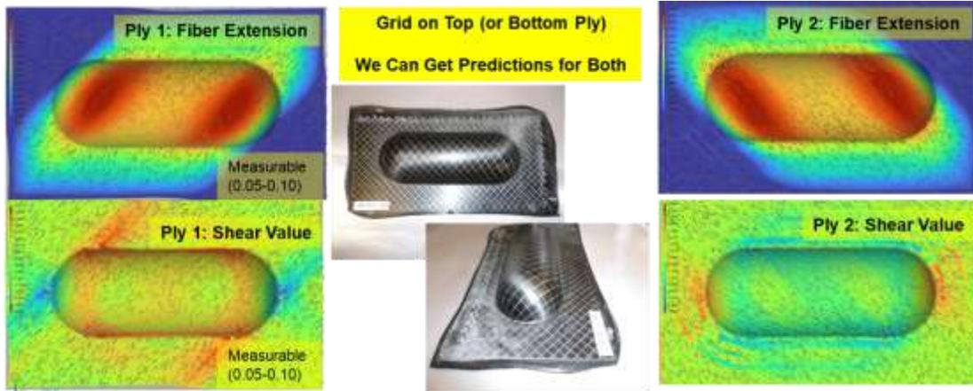
*Aniform model for +-45 degree bead during: Predicted deformation for each ply.*
