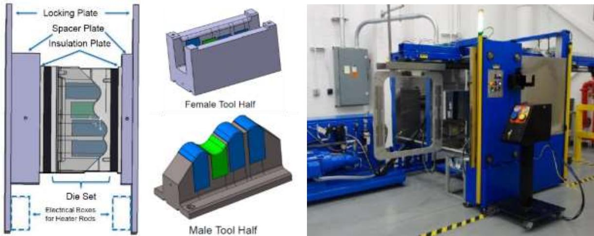
*Tool configuration for Vane forming demonstrations at Spirit (left, middle) and Thermoplastic Composite Forming Cell at Spirit.*
