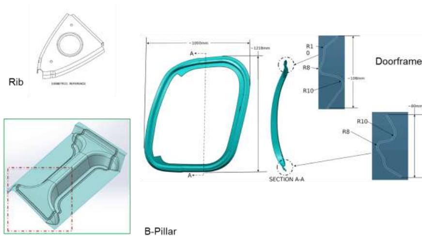
*Final part selection for Joby representing multiple levels of geometric complexity and combined features. Ribs represent the starting geometry, followed by the Door Frame and the Pillar.*
