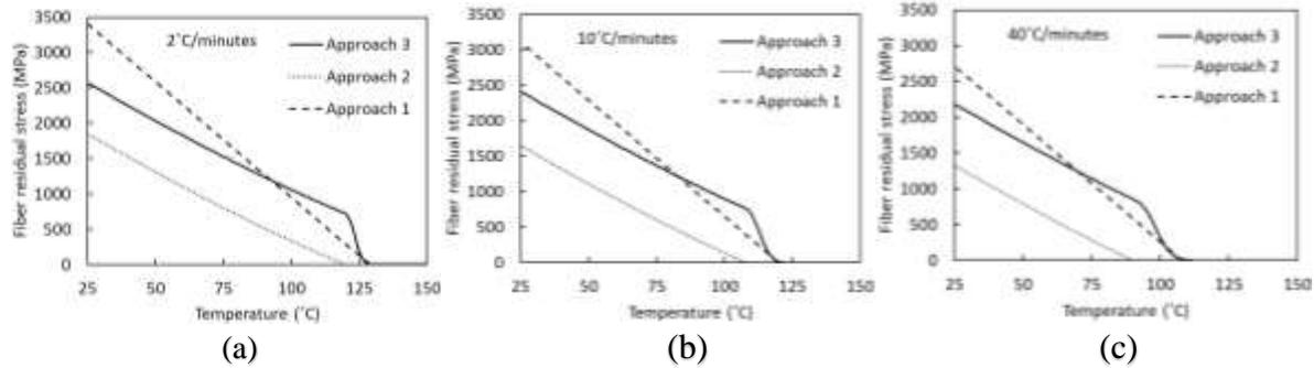
Axial residual stress at the mid-length of the fiber from  $T_m$  to  $T_{RT}$  (a) 2 °C/minutes (b) 10 °C/minutes and (c) 40 °C/minutes. All stresses are compressive.
