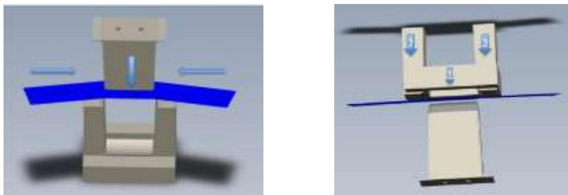
*Forming strategies for Vane geometry. Matched tool set on left works with tensioned blank to address draping at the bottom curve, two-piece tool set on right is a sequential process with matched forming of the curve, followed by tensioned forming of the walls.*
