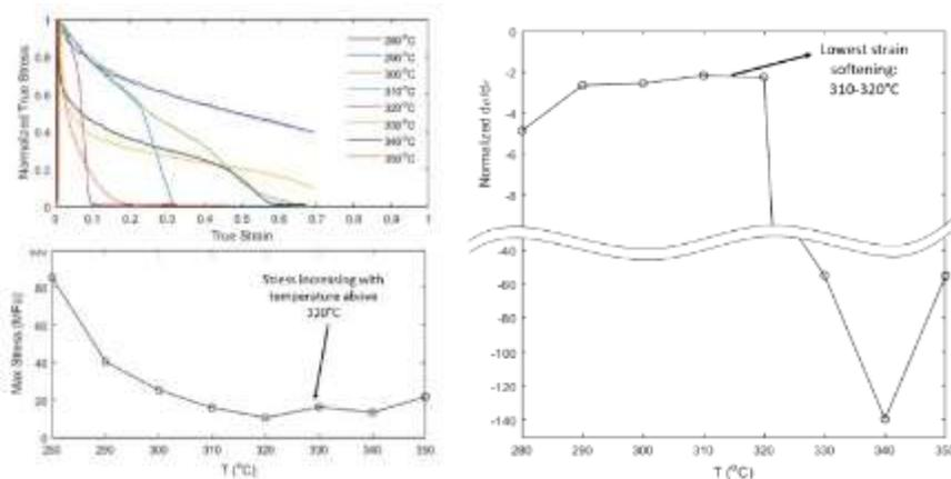
The normalized strain softening slope at the onset of viscous extension was between -5 and -2 for temperatures below 320C and abruptly decreases for temperatures 330-350C. Several other complex strain softening transitions are observed in the data as strain increases in different temperature ranges.
