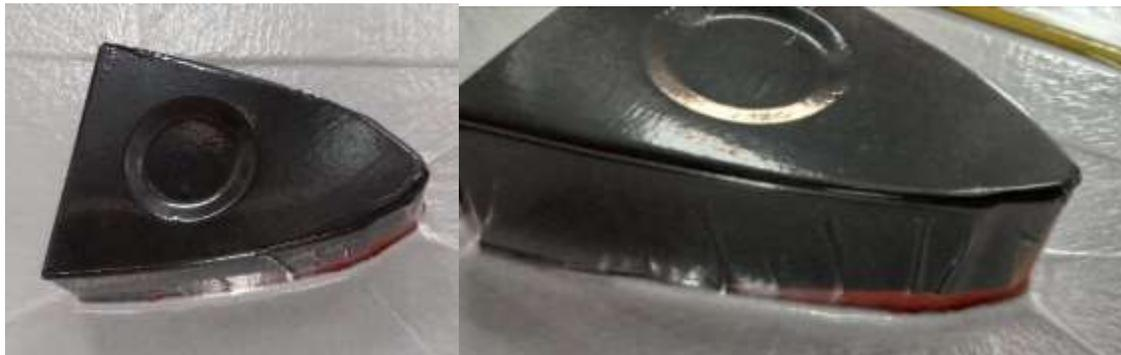
*Vacuum drape forming of Triangular Rib with flat debulked TuFF prepreg blank. TuFF stretch-forms the dimple, however wrinkles (right side photo) are seen on the curved flanges.*
