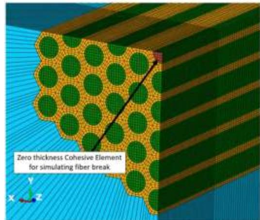
3D FE model with hexagonal packing of fibers.
