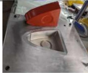
*Triangular Rib part detail and Tool. The Rib is a 4-ply design which is duplicated in TuFF prepreg blanks. A silicone male plug (in red) was cast to provide a male tool during forming and cure.*
