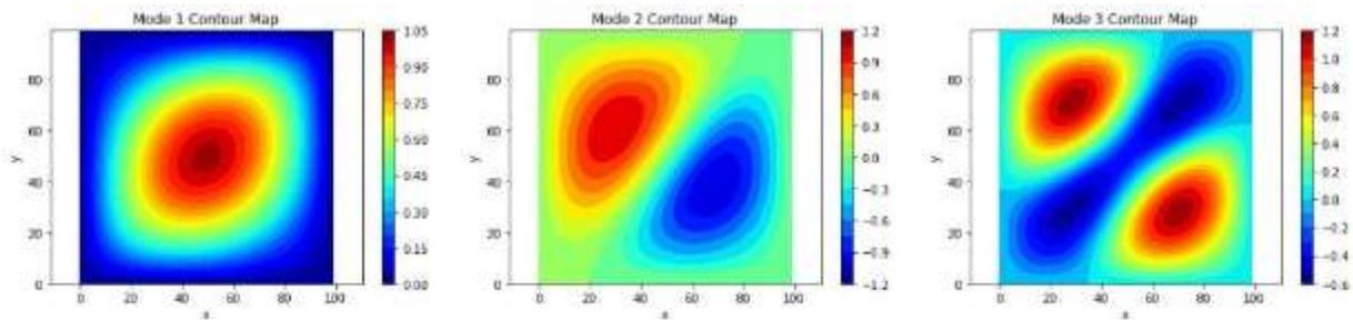
*Predicted first three modes of a simply supported graphite/epoxy  $[0_2/30_2/45_2]$  laminate under constant uniaxial loading.*
