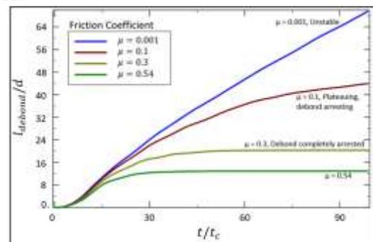
Debond growth vs. Time for elastic matrix with various coefficients of interfacial friction. The dynamic FE model simulation is stopped at  $t=165ns$  since the stress waves reach the boundary of the discretized domain.
