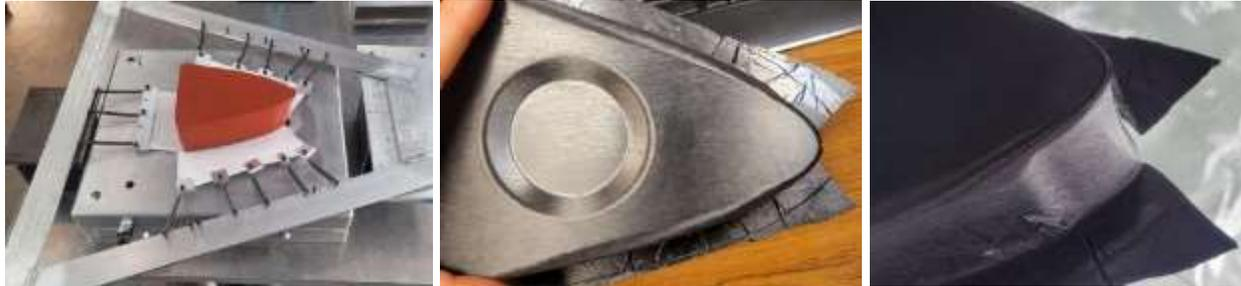
*Tensioned forming of Rib with TuFF prepreg blank. Tensioning frame/springs with prepreg schematic (left), Cured Rib showing surface dimple and joggled curved flange.*
