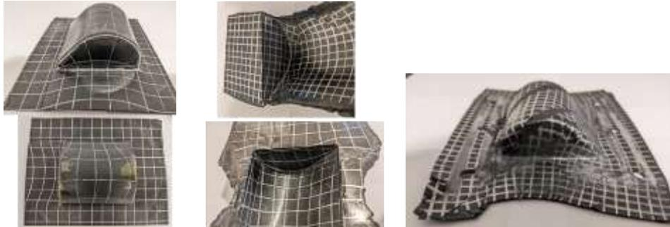
*Preliminary forming experiments under isothermal conditions to evaluate blank boundary effects on formed geometry for the bottom section of Forward Vane. Left is for fully clamped, middle is for no clamping and right is for multi-axial blank in clamped conditions.*
