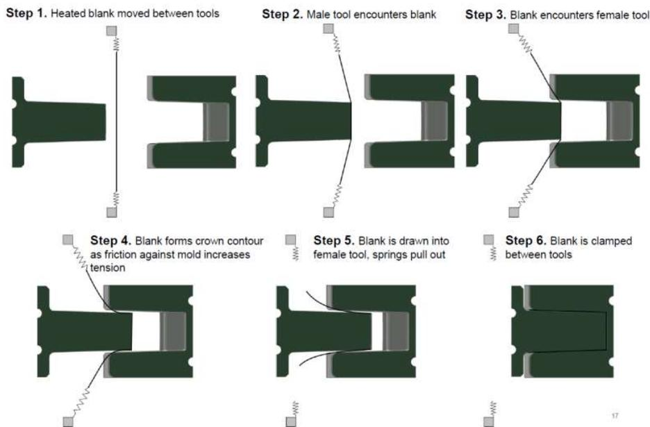
*Proposed initial forming methodology for Vanes. Process will be optimized based on formed Vane quality and initial trials.*
