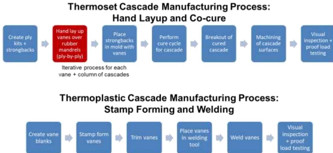
*Comparison of baseline continuous fiber cascade manufacturing process (hand layup and co-cure) with the proposed high-volume stamp forming process.*
