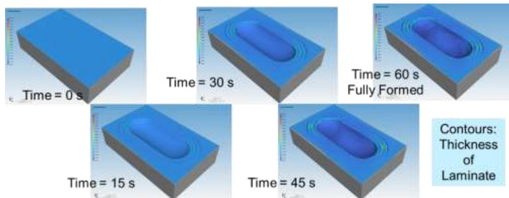
Aniform model for +45 degree bead during virtual forming
