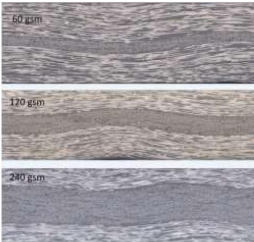
Most severe waves of fiber near the 90° layer with thicknesses ranging from 60 gsm to 240 gsm
