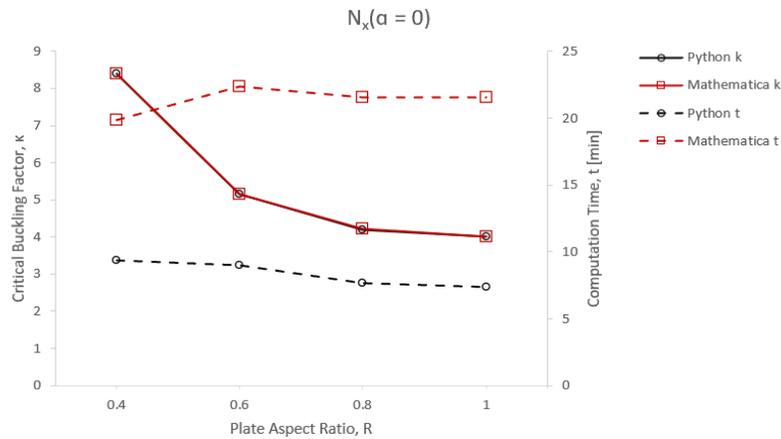
*Comparison of non-dimensional buckling factor between Mathematica and python program for a plate under constant uniaxial loading,  $N_x(\alpha = 0) = N_{crit} \left(1 - \alpha \frac{y}{b}\right)$ , with different aspect ratios.*
