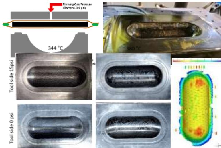
high temperature may be detrimental to forming. Samples were formed at temperatures of 344 and 380C. The results of the study show that the sample formed at 344C with a tool side pressure of 15 psi measured the highest uniformity in the strain pattern by photogrammetry.
