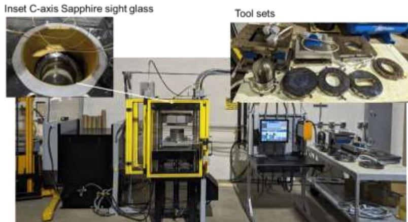
The hemispherical tool sets are designed to investigate deep drawing and tool ply interaction. The flat tool sets are design for imposing defined strain modes
