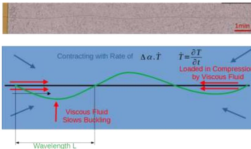
*Forces and Geometry of Fiber Bending in Contracting Fluid*
