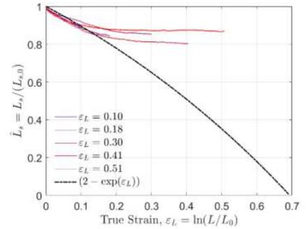
The conclusions from this micromechanics model are that fiber spacing distribution will contribute to an order of magnitude increase in the measured extensional viscosity, the fiber spacing will not relax during deformation, and that fiber overlaps in the microstructure will recover during extension. This recovery of fiber overlaps is the primary mechanism for ply thinning during stretch forming (reported in the previous year).
