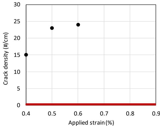
Matrix crack density in 90° plies of [0/90/0] laminate at ~1 million cycles. Continuous IM7/K3B (black dots) exhibits a crack density of 25/cm. In comparison, 3mm IM7/LM-PAEK cross-ply (red squares) exhibits zero crack density (does not microcrack at strains less than 0.9% strain). Our plans for the coming year will focus on fatigue testing of the cross-ply laminates with reduced ply thickness (once the process has been optimized to reduce layer waviness) at higher strain levels.
