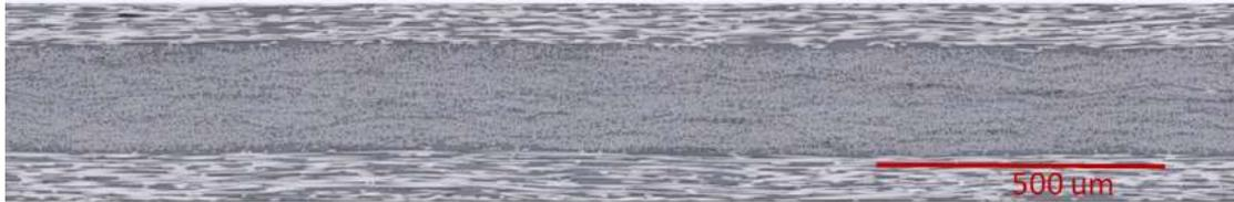
Cross-section of [0/90/0] IM7/LM-PAEK TuFF cross-ply laminates with a thick 90° ply areal weights of 240 gsm. No transverse cracking is observed after fatigue at 0.9% (R=0.1)
