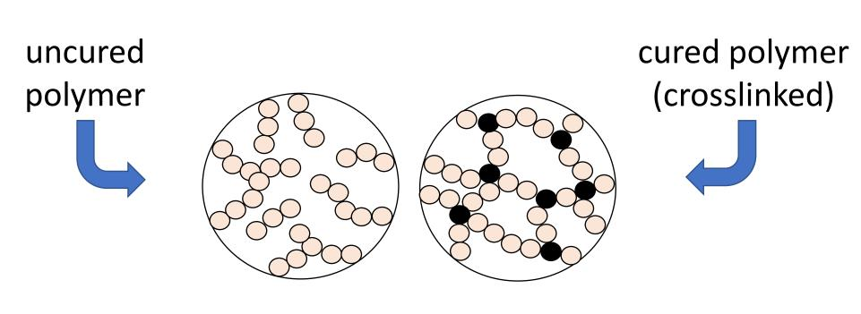
When a thermoset cures, the polymer crosslinks. Crosslinking is the connection of polymer chains. Crosslinking changes the properties of the polymer making it stronger
