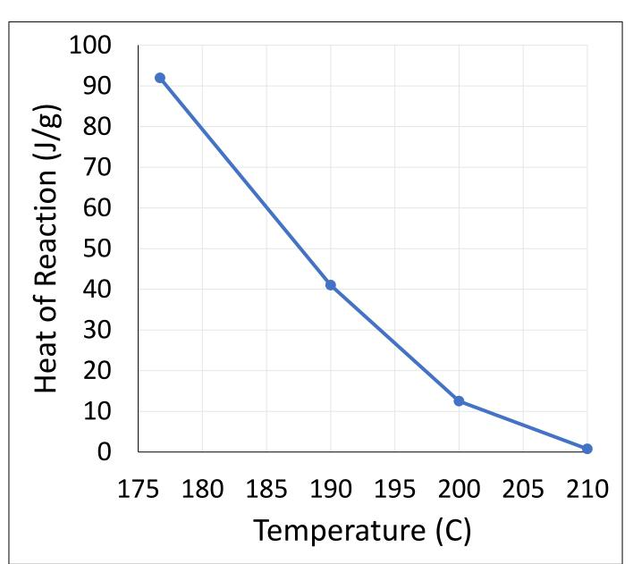
The first graph shows the peak of the degradation from the TGA overlaps the DSC data. From the first graph, the convolution of peaks affecting the residual heat of reaction is shown. The residual heat was found after running cure cycles with different isothermal hold temperatures for 6 hours. The relationship of residual heat of reaction against temperature is shown in the second graph. As the temperature increases for the isothermal hold temperature, the residual heat of reaction decreases.
