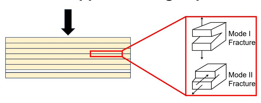
To improve resistance to interlaminar failures in the composite, interlayer toughening is utilized to reduce shear stresses through decoupling of plies increasing delamination resistance.
