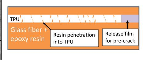
Hypothesis: RDL-RDC resin properties change at elevated temperature to allow more diffusion, comparable to that of SC-15 Resin at room temperature.
