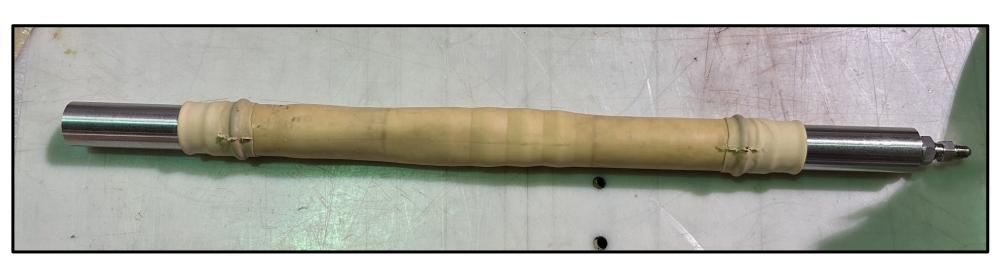
After bladder molding the prototype, the tool successfully disassembled from within the bladder for extraction
