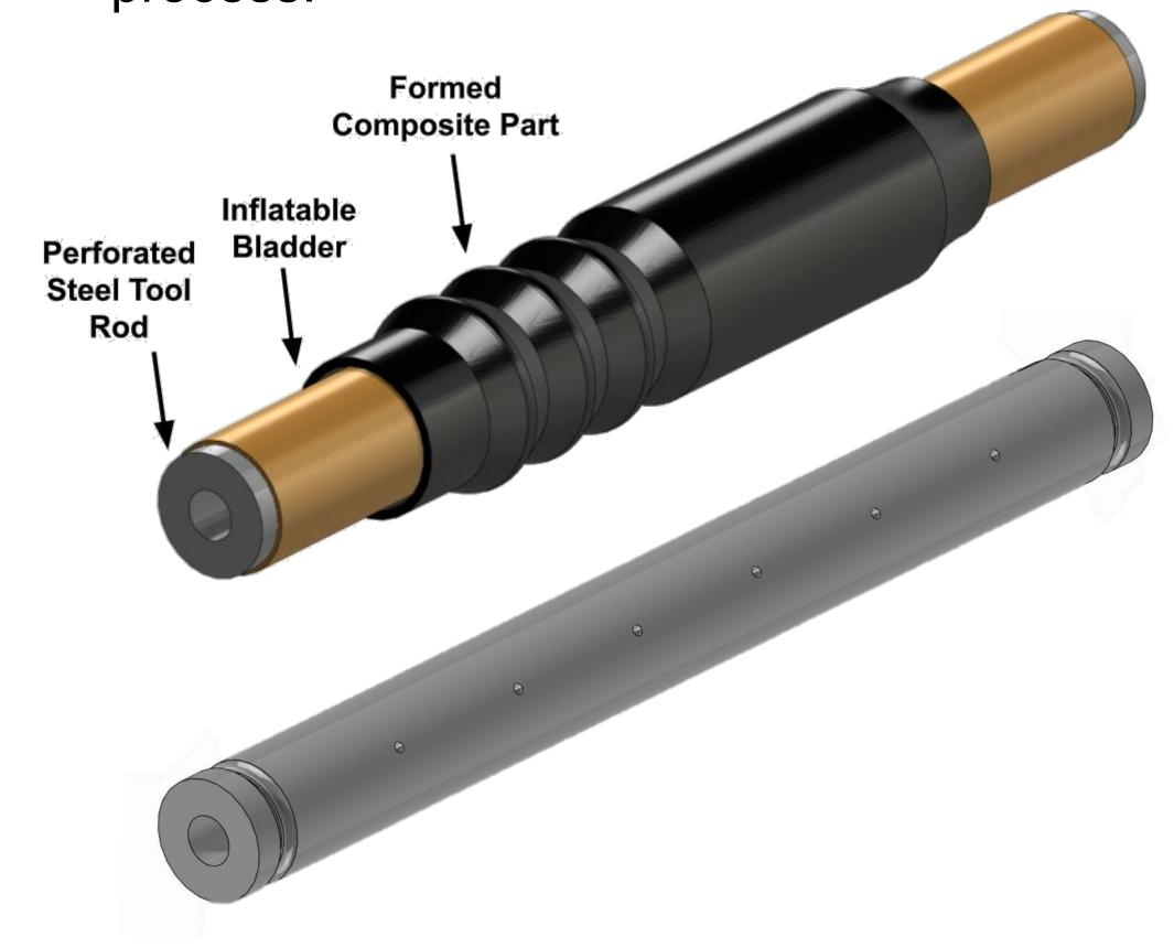
The tool core is used as a structure for laminating the composite.
