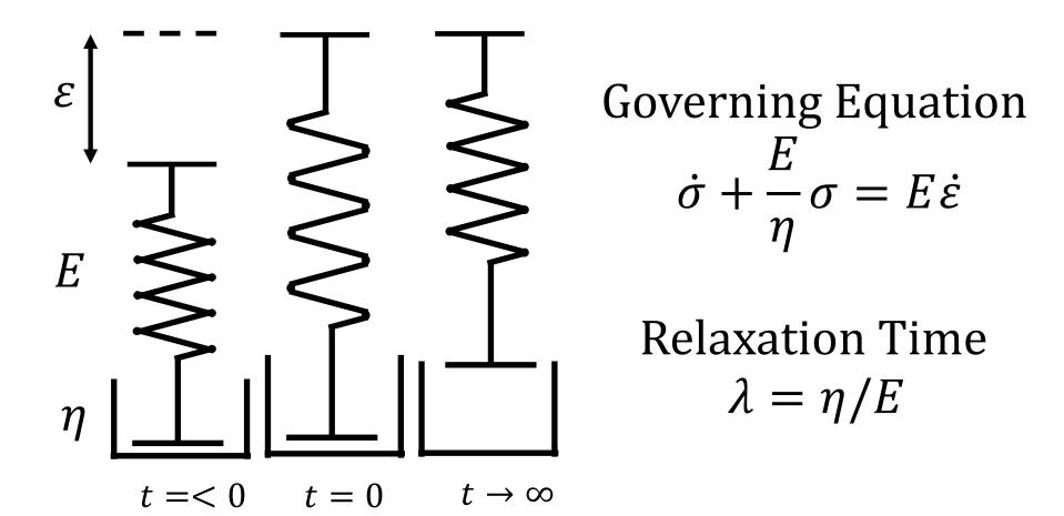
The model can be solved for loading under constant strain rate or stress relaxation at zero strain rate. Both test methods can be implemented to determine material properties.
