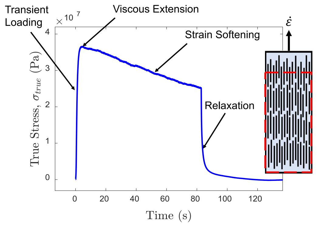
Previous work has focused on the viscous response of the material for loading under constant processing conditions  $(T, \dot{\varepsilon})$ . This established a power law trend for viscosity  $(\eta)$  consistent with shear thinning polymers.
