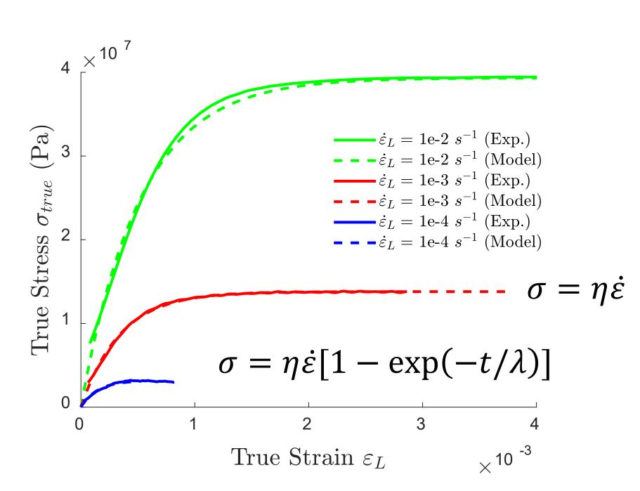
The Maxwell model was fit to the initial loading to determine the relaxation time. An Arrhenius shift was applied to the data to relate all samples to a common temperature of 330°C.
