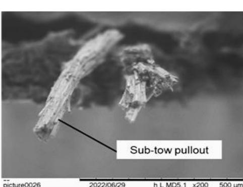
Composite failure mode SEM image
