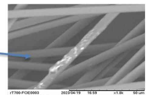
GLO depolymerization of Elium is successful with >95% fiber reclamation with minimal property degradation and residue on fibers
