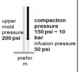
Enables infusion of High FVF TuFF preforms maintaining 200 consolidation PSI while pressure
