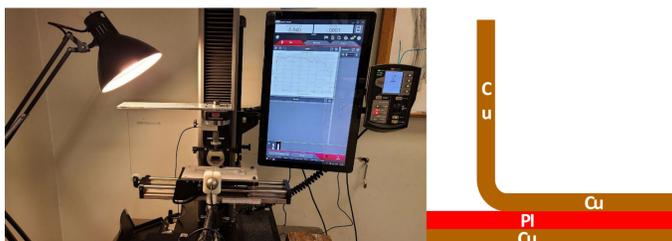
90-degree peel test → Photograph and schematic of a 3-layer Cu-PI-Cu specimen provided by DuPont
