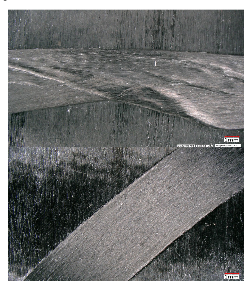
Fig. 3: 100 mm steering; wrinkles in continuous tape (top), wrinkle-free TuFF (bottom)
