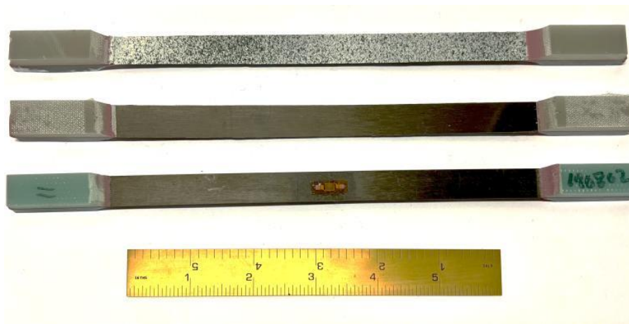
Figure 4. TuFF test specimens, DIC speckle coated (top), back side (middle), strain gauged back (bottom).
