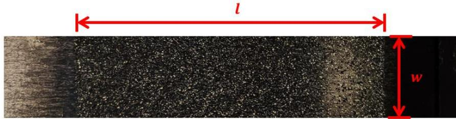
Figure 2. Prepared TuFF samples after cutting and speckling, with a speckled length and width of 3" and 1" respectively. After a drying cycle, the samples are ready to be tested.
