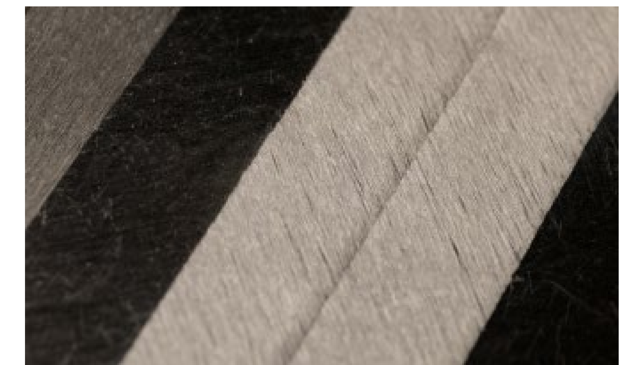
250gsm quasi-isotropic [0/90/45/-45]s laminate
