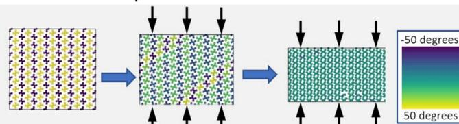
Change in morphology in polyethylene (PE) crystal under transverse pressure (color coded based on the angle of the chains).
