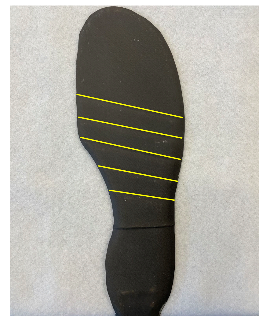
Rocking motion layup made in the footplate
