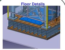
Sandwich construction with 6 120"x30"x1" Floor plates &10 x 10.5"x 5.85" W F beams
