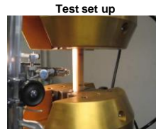
Shown with camera setup to manually track crack growth
