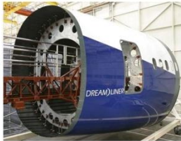
Composite fuselage section of the Boeing 787 Dreamliner. Photo Credit: Boeing Photo
