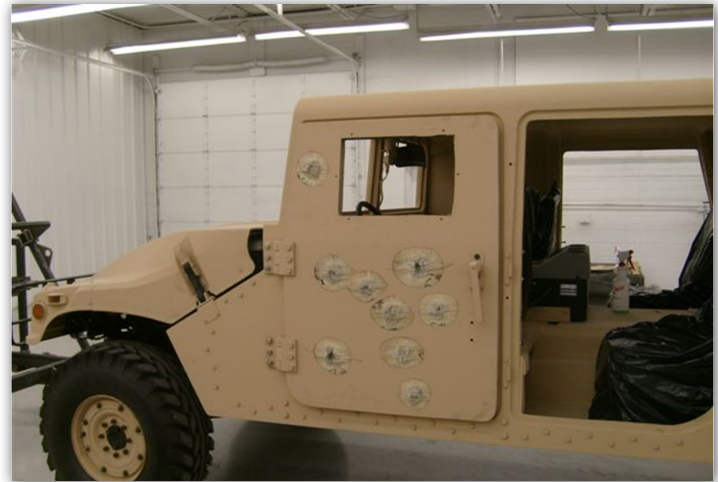
ACMV #3 – Driver’s door is the ballistically tested UD-CCM composite armor door
