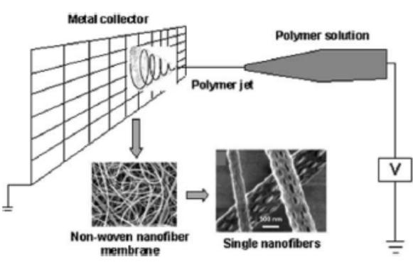
High surface area and high aspect ratio of the nanofibers are very important parameters determining unique properties of these materials.
