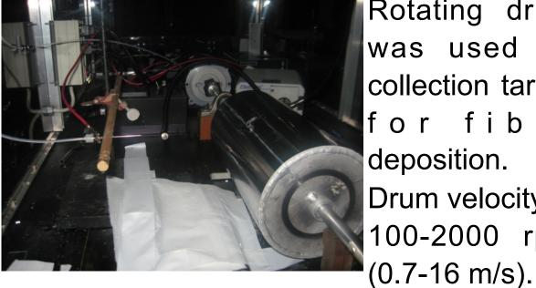
Rotating drum for fiber 100-2000 rpm 100 rpm
