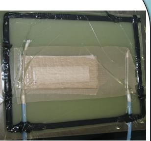
The feasibility of conventional VARTM technique for the fabrication of the epoxy-based composites reinforced with electrospun fibers was experimentally verified in this work.
