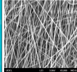
Nylon 6,6 was spun from the mixture of formic and acetic acid at 1500 rpm (~12 m/s). Average fiber diameter: ~100 nm Polar solvent induces jet instability during electrospinning process lessening fiber alignment. However, uniaxial orientation of fibers is not necessary for toughening applications in composites.
