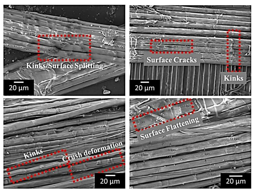
Understand **Project statement:** processing-induced damage occurring at the crystalline level
