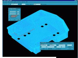
Simulating Controlled Injection Into Complex Part
