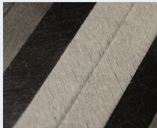
250gsm quasi-isotropic [0/90/45/-45] s laminate
