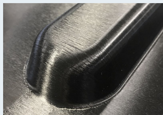
250gsm quasi-isotropic [0/90/45/-45] s laminate
