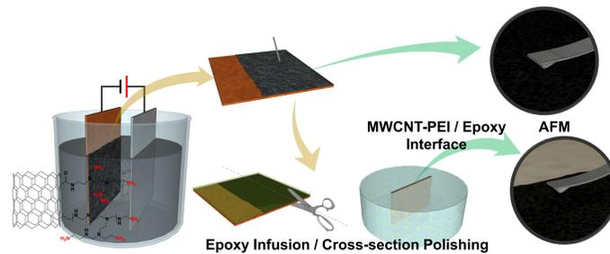
**Electrophoretic deposition** of PEI functionalized MWCNTs on copper tape, mimicking the nanocomposite films at fiber-matrix interface of hybrid composites.
