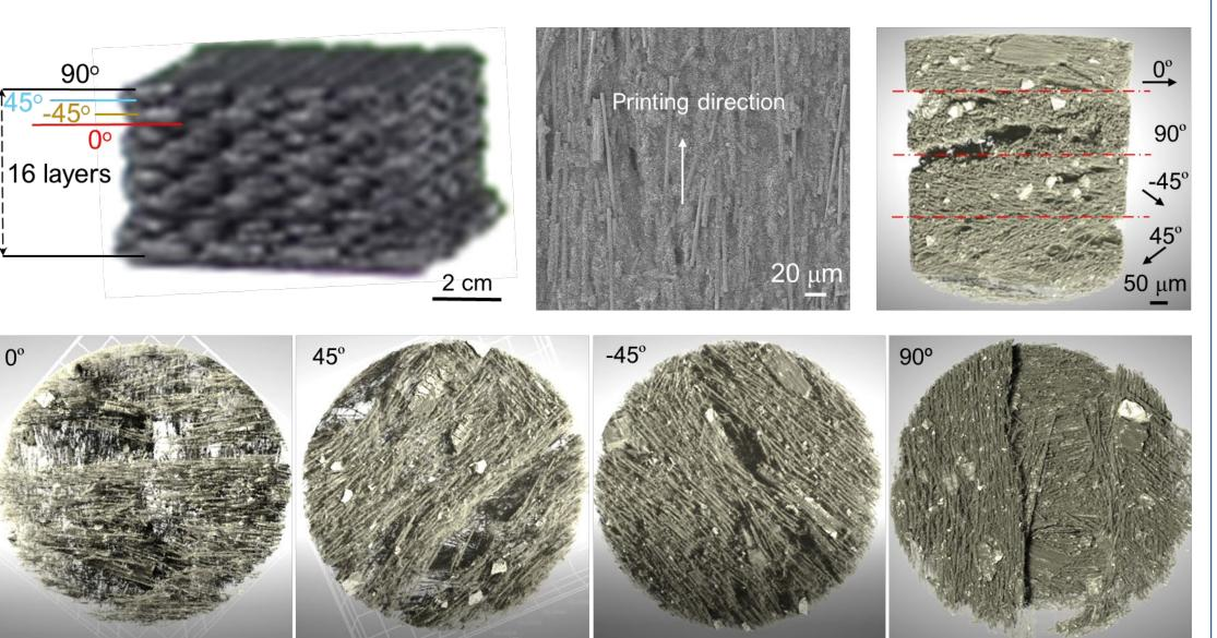
The rCF/PLA sample remains structurally stable during the "green-to-brown" transition with heat applied.
