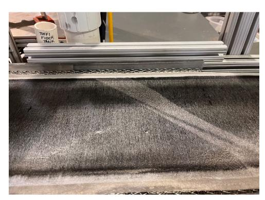
90 Minute burn-off processing significantly reduced clumping in the batch and pyrolyzing processing removed remarkable amount of residue
