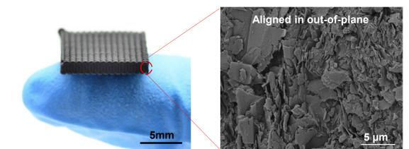
3D printing has the potential to fabricate structured electrodes on a large scale. As a laboratory-scale demonstration, single-sided electrodes were made by co-sintering electrodes/current collectors.
