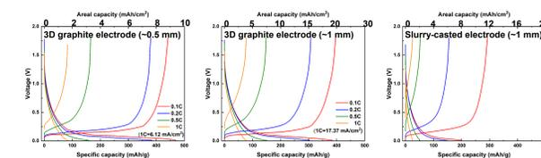
The 0.5mm thick structured electrode delivered the highest specific capacity of ~ 80 mAh/g at 1C. On the other hand, the slurry-casted electrode delivered a much lower capacity of ~ 25 mAh/g at 1C.
