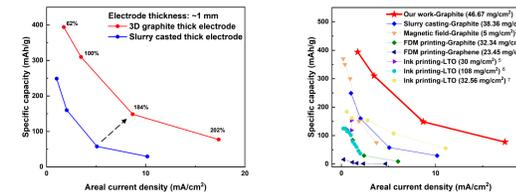
As the current density increases, the performance gap increases, more than doubling at 1C. Our 3D printed structured electrodes have high electrode material loadings and can achieve highest capacity due to the aligned graphite structure
