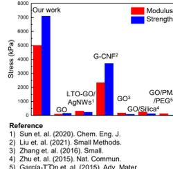
The structured electrode has higher compressive properties than the other reported 3D printed electrodes, showing good structural stability.
