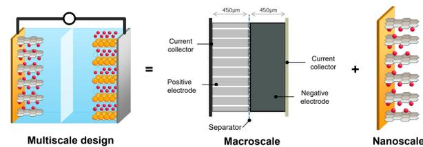
3D printing can rapidly fabricate structured electrodes with an out-of-plane aligned architecture with low tortuosity and mechanical robustness.
