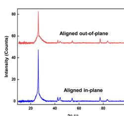
Tracking the intensity of the (002) Bragg peak corresponding to the graphite basal plane reveals the out-of-plane-alignment of graphite.
