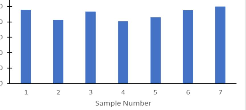
experimental IFSS of the resinmatrix was determined to be 55 MPa with an STD of 7.35
