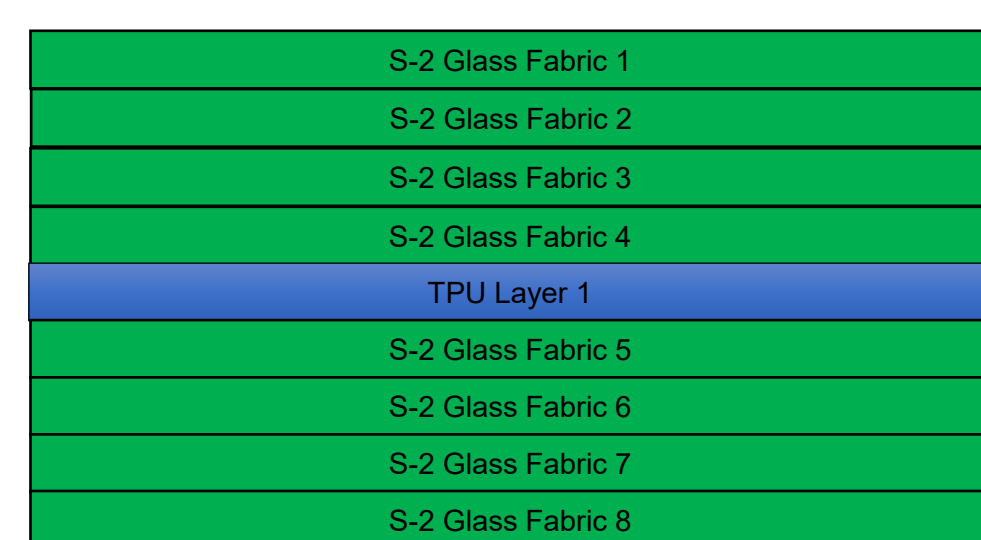
Fig: Layup with 8 S2 glass fabrics with one layer of TPU in between
