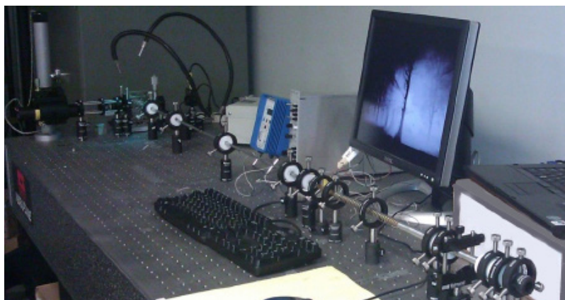
High strain rate dynamic microdroplet test
