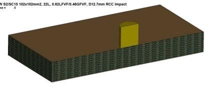
$V_I$  = 932 m/s Impact on 22 Layer Plain Weave Glass/Epoxy Composite
