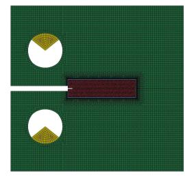
$V_I$  = 200 m/s Impact Local Tow-tow Delamination and Cone Wave Initiation
