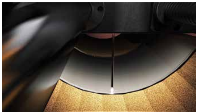
A simplified rendering of the CSAM process concept for fabricating an SS pipe inside an aging pipe
