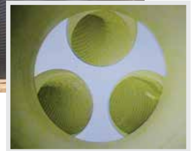
Dust collector with three 16-inch hoses was used to recover leftover cleaning grit
