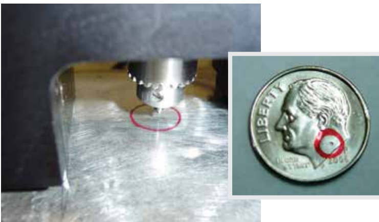
Figure 3. Indentation shown to scale on a dime. Each test is performed in under five minutes
