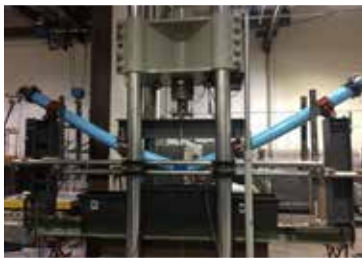
Figure 2. Physical testing of pipe infrastructure at CUB CIEST
