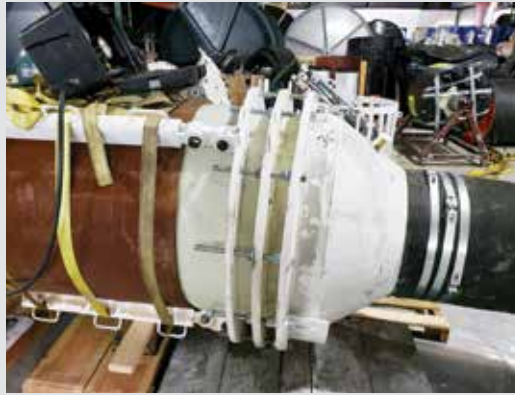
Extensive shop testing of the Guide Pipe and Reducer configuration ensured that the liner would traverse the obstacles and invert properly over the entire length of “The Mess”
