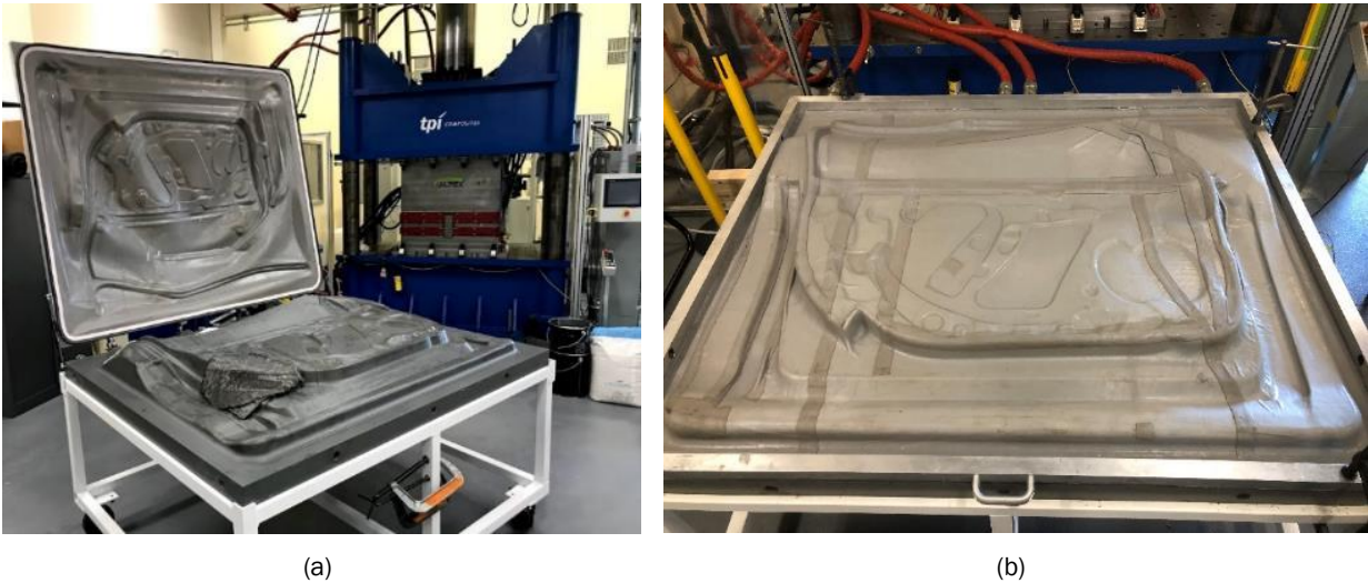
Figure II.2.3.14. Al preform tool with the silicone vacuum bag in (a) the open position and (b) the closed position. Source: TPI Composites.
