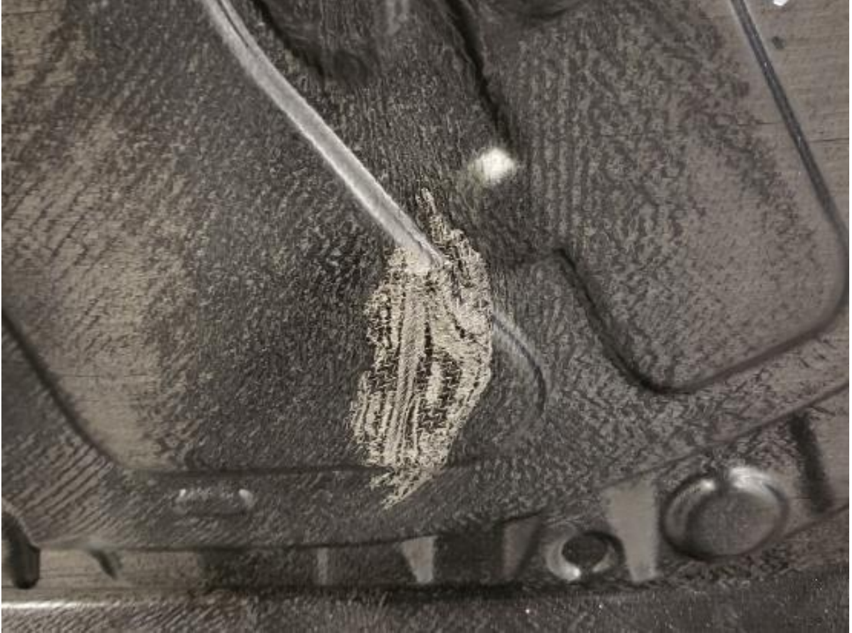
Figure II.2.3.20. Dry area. Source: TPI Composites.
