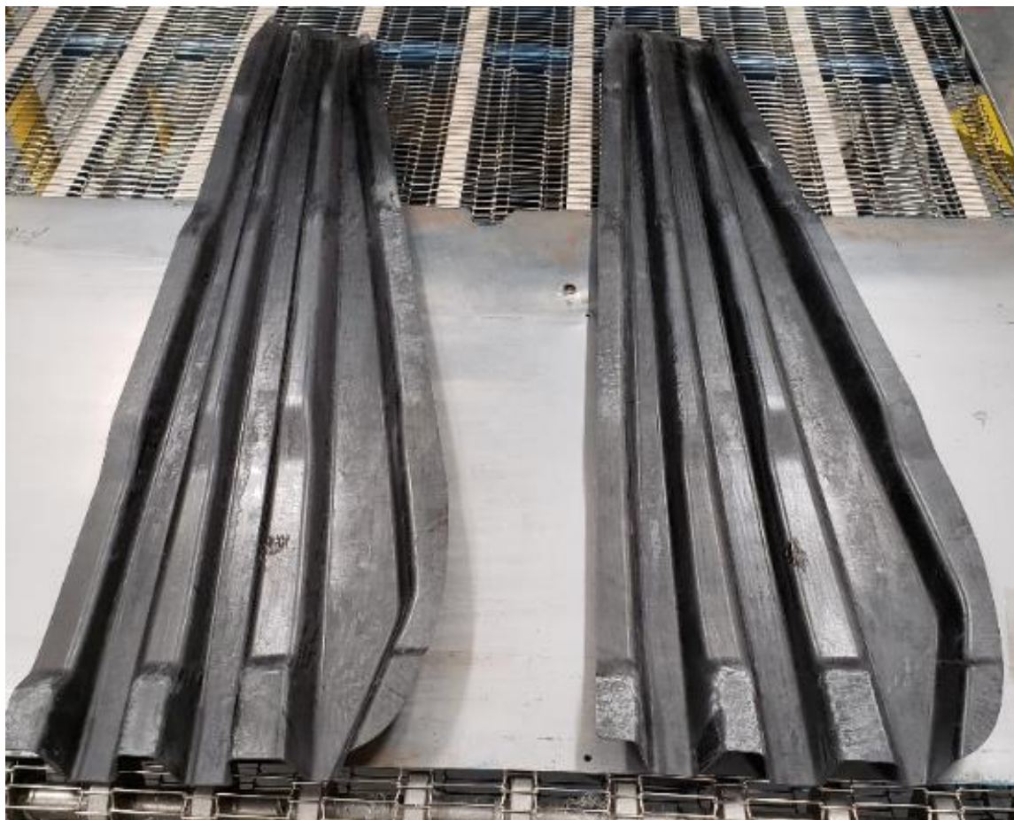
Figure II.2.3.18. HP-RTM molded intrusion beam hats. Source: TPI Composites.
