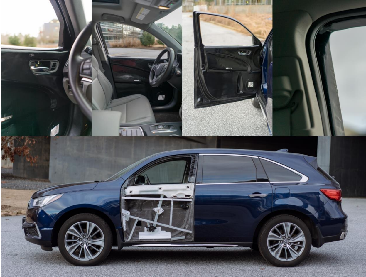
Figure II.2.4.17. Fully assembled door frame on the existing vehicle. Source: Clemson University.
