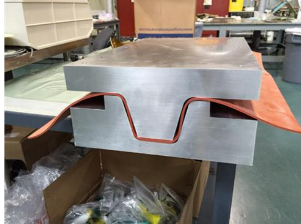
Figure II.2.4.6. Subcomponent tool for hat production. Source: University of Delaware.
