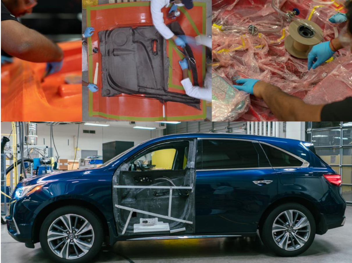
Figure II.2.4.16. Composite door manufacturing process. Source: Clemson University.
