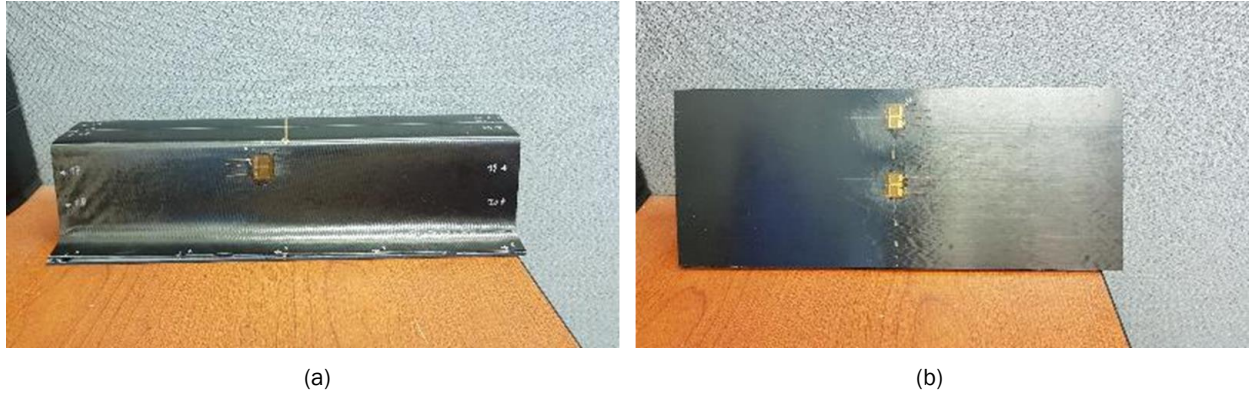
Figure II.2.4.13. Location of the bonded strain gauges on (a) the side and (b) bottom in order to record strain during impact. Source: University of Delaware.
