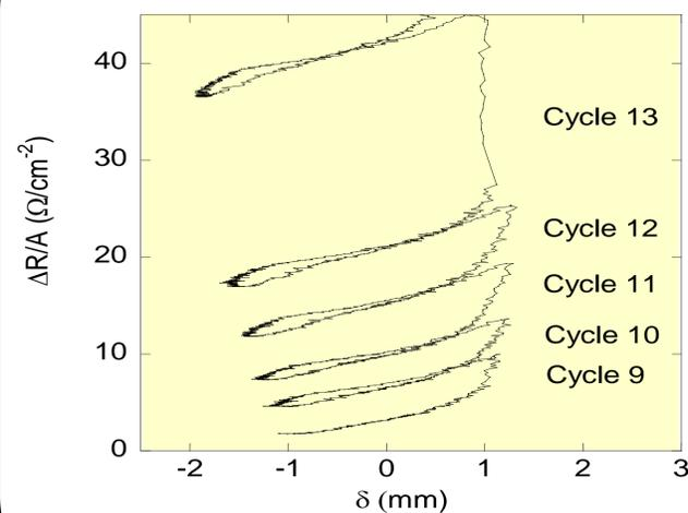
◆ New crack formation, and hysteresis are apparent in the resistance / deformation behavior.
