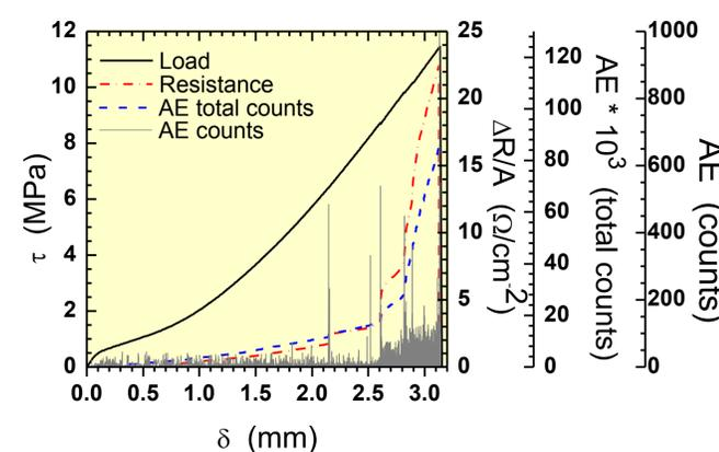
Composites are processed with a high void content are used to promote composite failures. The damage sustained at higher extensions corresponds to fiber breakage and ply delamination.
