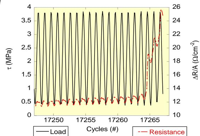
◆ Specimens fatigued to failure show the sensitivity of the sensing capabilities; note the upward trend of the resistance baseline prior to failure.
