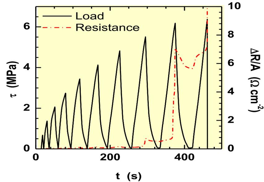
◆ As observed in the tensile composite failure, minimal damage is sustained at lower stress levels. At stress levels prior to failure, the corresponding fiber breakage leads to rapid increases in damage.
