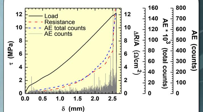
Progressive damage accumulation at lower extensions suggests damage to the adhesive, while the rapid increase in damage represents damage at the composite interface.
