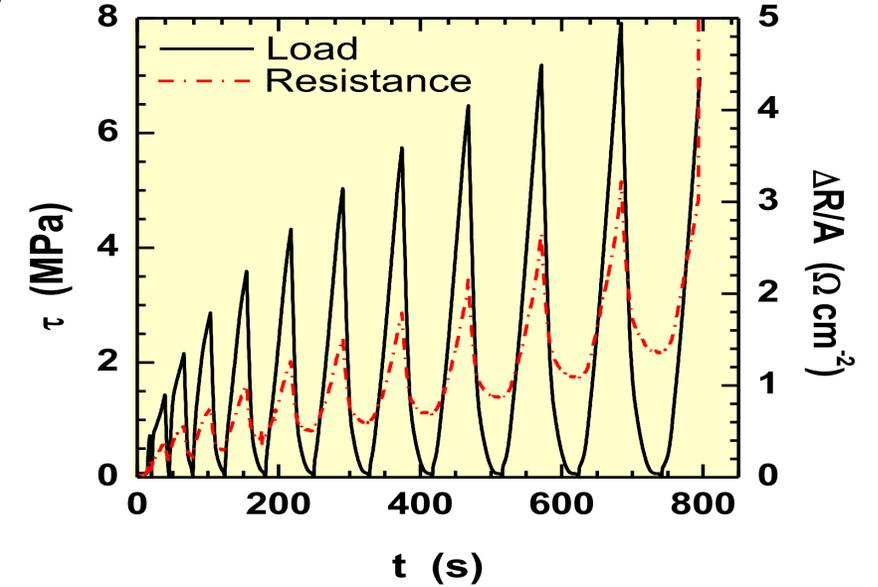
◆ The resistance behavior of combined failures for cyclic testing is similar to that of the tensile case, with the progressive damage accumulation throughout the test.
