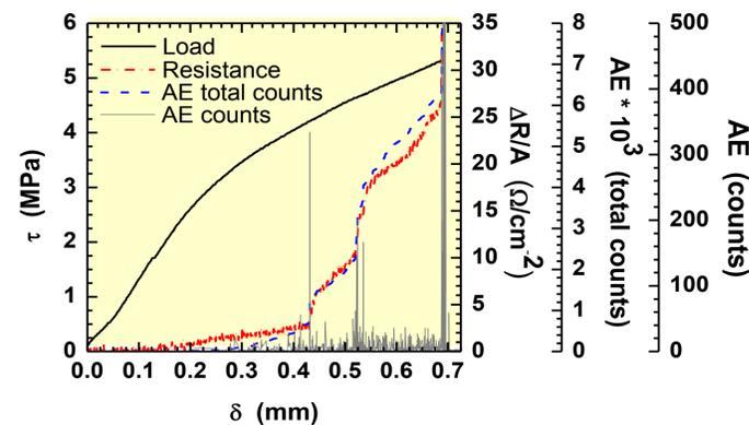
During tensile loading, the damage in the Hysol joint is reflected in the increasing change in resistance and total Acoustic Emissions (AE) as the CNT network in the adhesive is destroyed. The jumps in damage represent debonding between the epoxy & steel.
