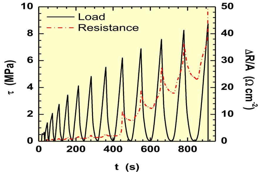
◆ The baseline resistance behavior is similar to that in the tensile test for this failure mechanism, with distinct regions of increased damage accumulation throughout the cycles.
