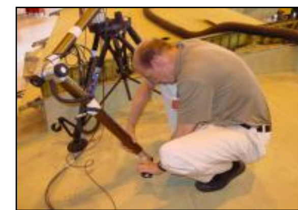
FARO Arm Scanned Part into CATIA
