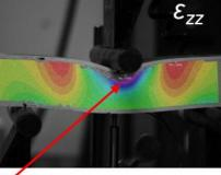
Core crushing / local compressive failure
