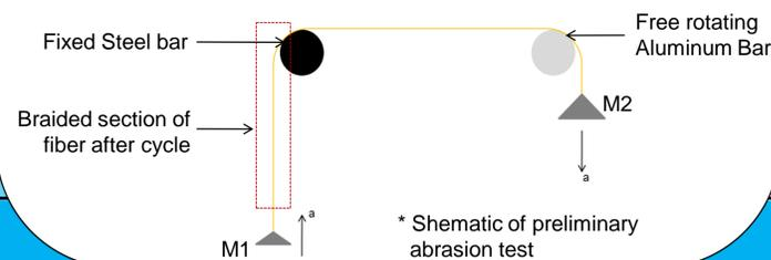
\* Schematic of preliminary abrasion test
