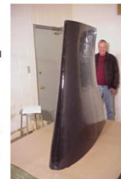
¼ scale twisted rudder manufactured by Production Products
