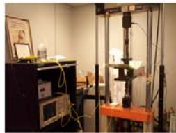
3-point bend test performed using 1550nm light source fed through each fiber with an optical spectrum analyzer displaying the wavelength
