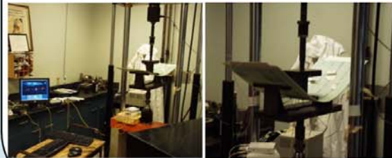
3-point bend test performed using 1550nm light source fed through each fiber with an optical spectrum analyzer displaying the wavelength
