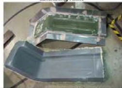
Cure overnight and then pull the mold from the original part.
