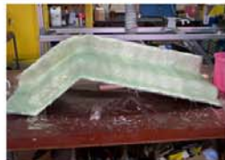
Cover tooling dough with a layer of glass fabric and laminating resin.
