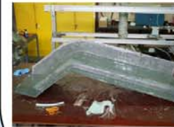
Apply glass fabric and laminating resin.
