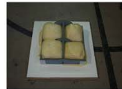
Fill with expanding urethane foam.
